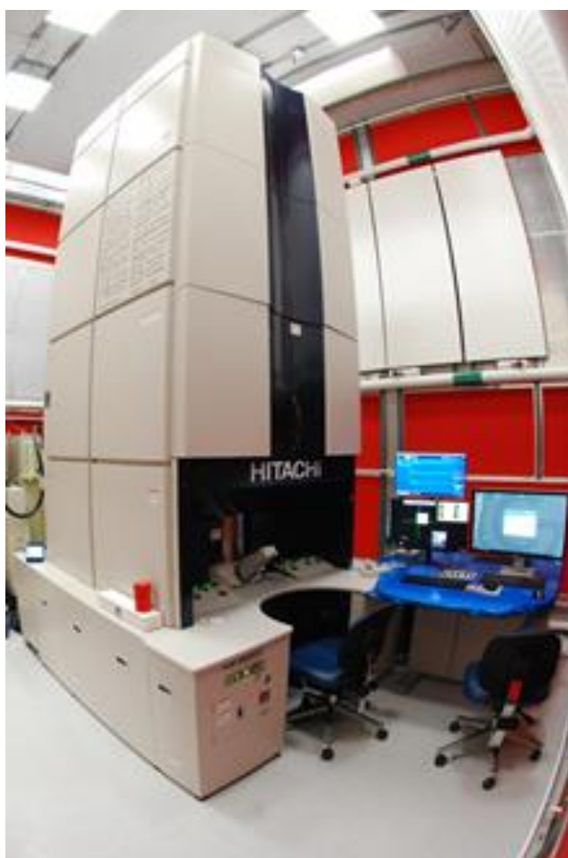
Figure 2. Column length of the Hitachi HF3300 (S), illustrates one of the challenges for engineering design for instrument stability and room design specification.
